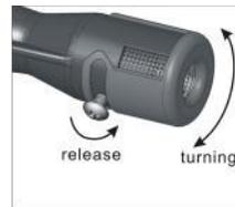
1. Release the screw on venturi tube.
