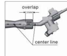
1. Overlap 20 mm between venturi tube and nozzle when assembly.
