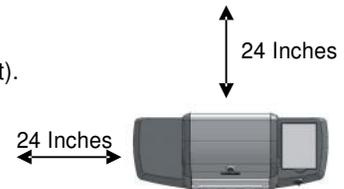
Always locate this grill where there will be ample combustion and ventilation air, but never position it in the direct path of a strong wind.
