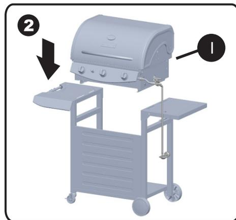
3) Install the grill housing assembly using **six** washers (GG), lock washers (HH), and M6x12mm screws (BB) as shown. First insert the back screws in an alternating pattern (install one screw on the left then install the next screw on the right side).
