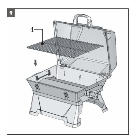
**Step 9**Put the cooking grid onto the heating plate as shown.
