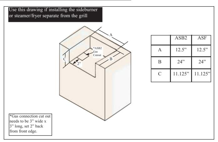
If installing the Steamer/Fryer (ASF), the Gas Cutout needs to be located on the right side of the built-in island, opposite the sideburner location.
